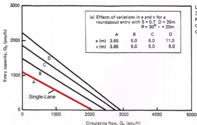
Line A is for Single-Lane ( $V = 3.65\text{ m}$ ,  $E = 3.65\text{ m}$ ) from Kimber LR 942, 1980. This capacity line closely matches original NCHRP data.
