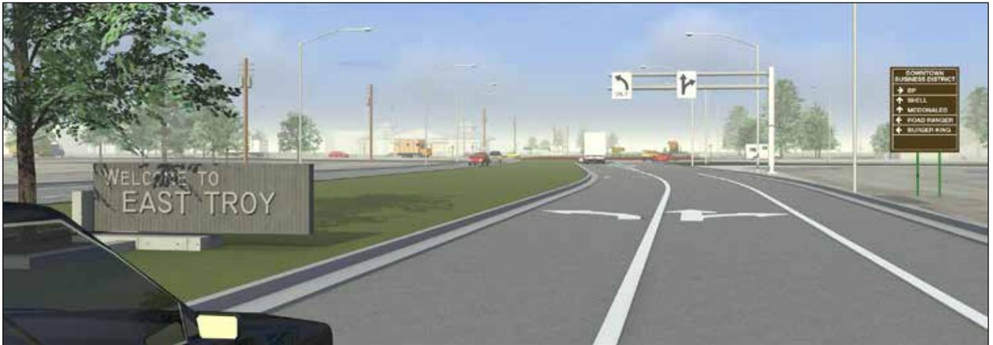
When intersection improvements are planned, the operational requirements of signalized intersections (storage lengths, speeds, etc.) require business access drives to be reduced, restricted and even removed. Roundabouts, on the other hand, provide significant flexibility for the spacing and location of business driveways without the safety and operations issues associated with the same access at signalized intersections.
