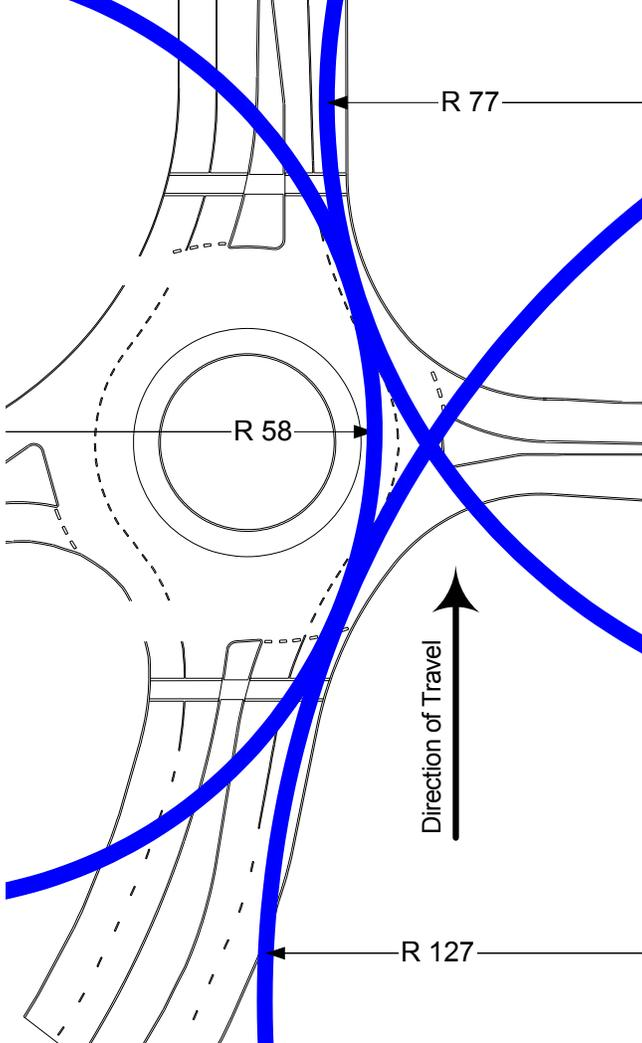
**Figure 3. Fastest Path Approximation for Small Urban Roundabout.**
