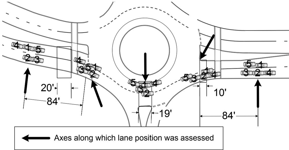
**Figure 1. This Scale Drawing of the Small Urban Roundabout Depicts the Mean Lane Position for Each of the Five Identified Groups.**
