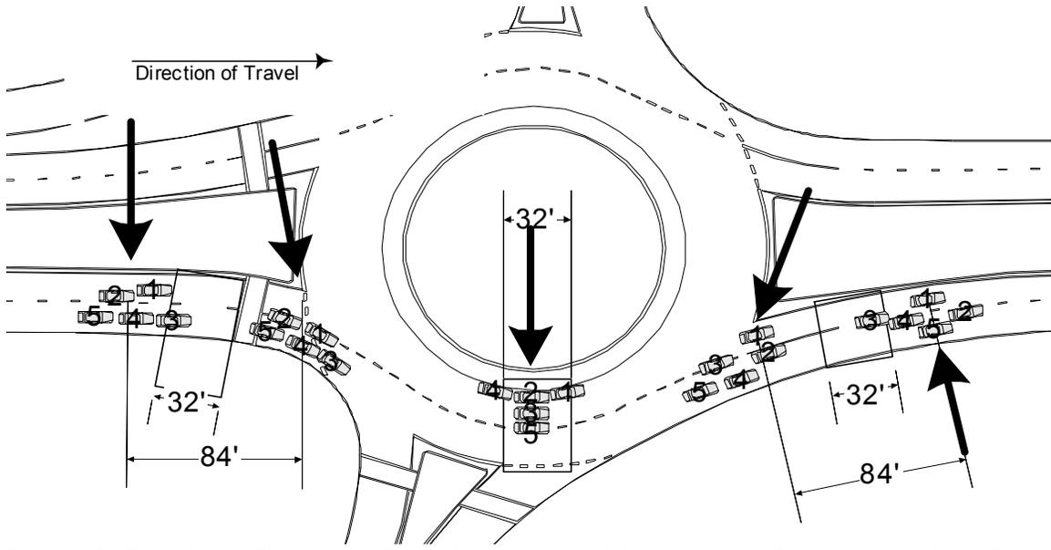
**Figure 2. This Scale Drawing of the Interchange Roundabout Depicts the Mean Lane Position for Each of the Five Identified Groups.**
